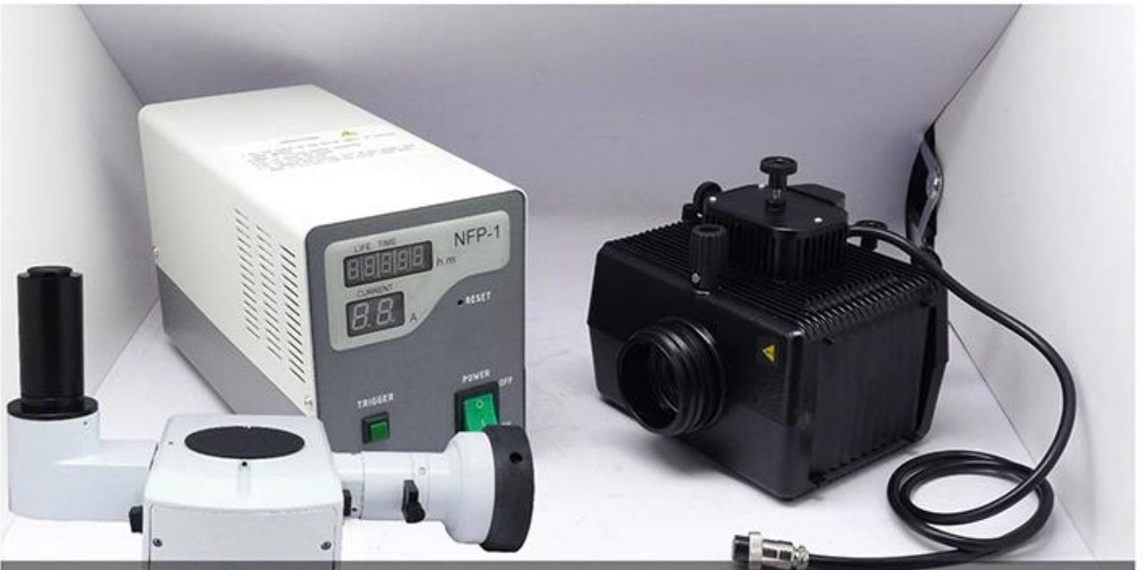
SLV-SZ68F EPI-Fluorescent Attachment For Stereo Microscope
